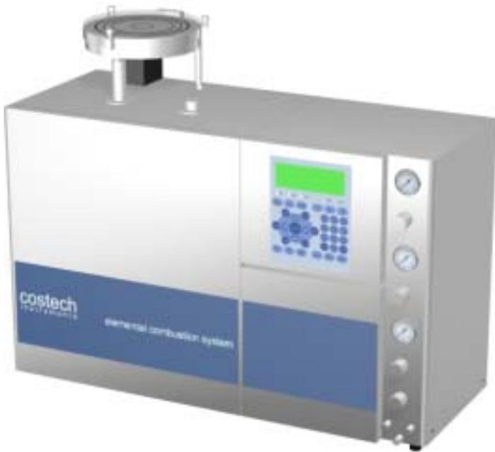
to signal detection - is microprocessor controlled. It represents an evolution in the technique of elemental analysis by "flash combustion/ chromatographic separation and multi-detector techniques".
